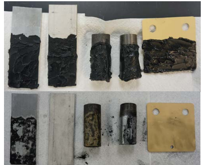
Lab testing of various metals with Br-PAC
